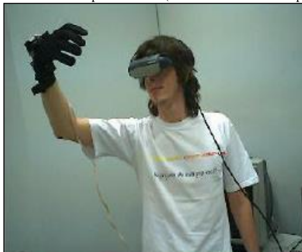
Figura 4 – RV Imersiva com capacete HMD (Helmet Mounted in Display – Capacete)
