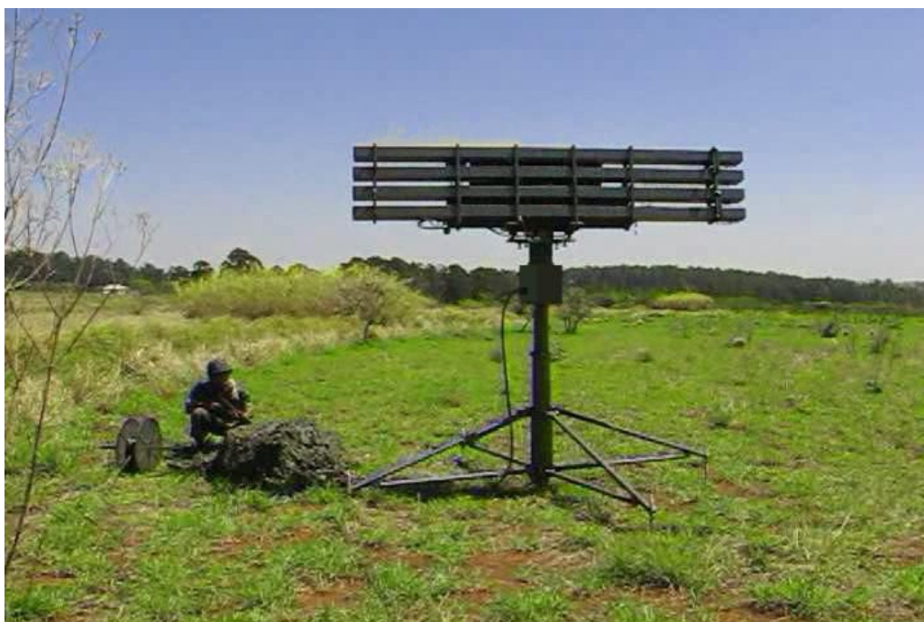
Fig. 6 – Radar SABER M 60
