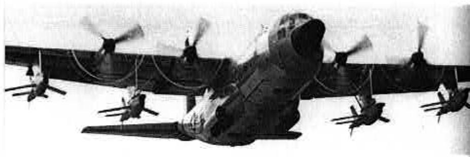
FIG 4.1 VANT Lightning Bug
