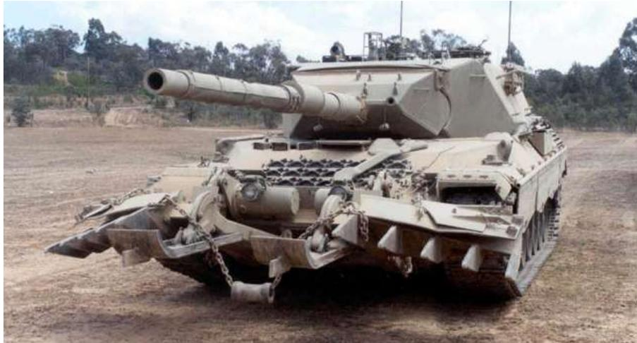
FIGURA 6 – Track Width Mine Plough (TWMP)
