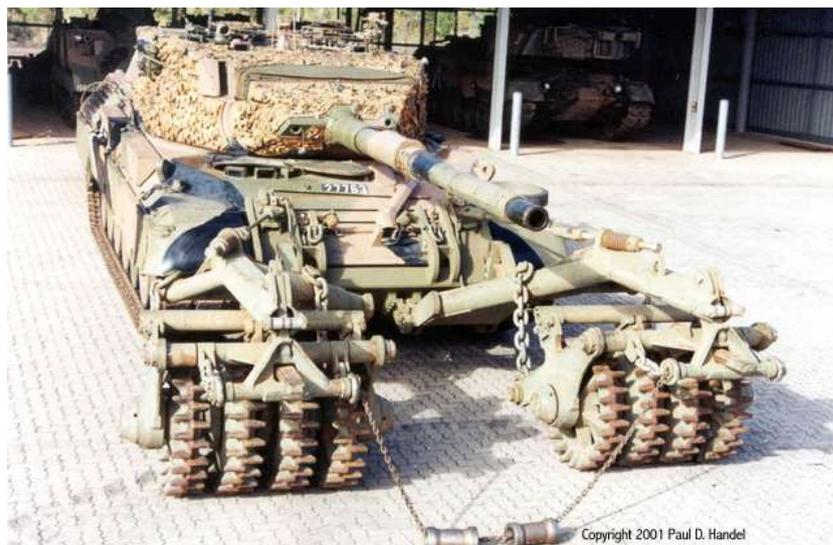
FIGURA 7 – Mine Clearing Roller System (MCRS)
