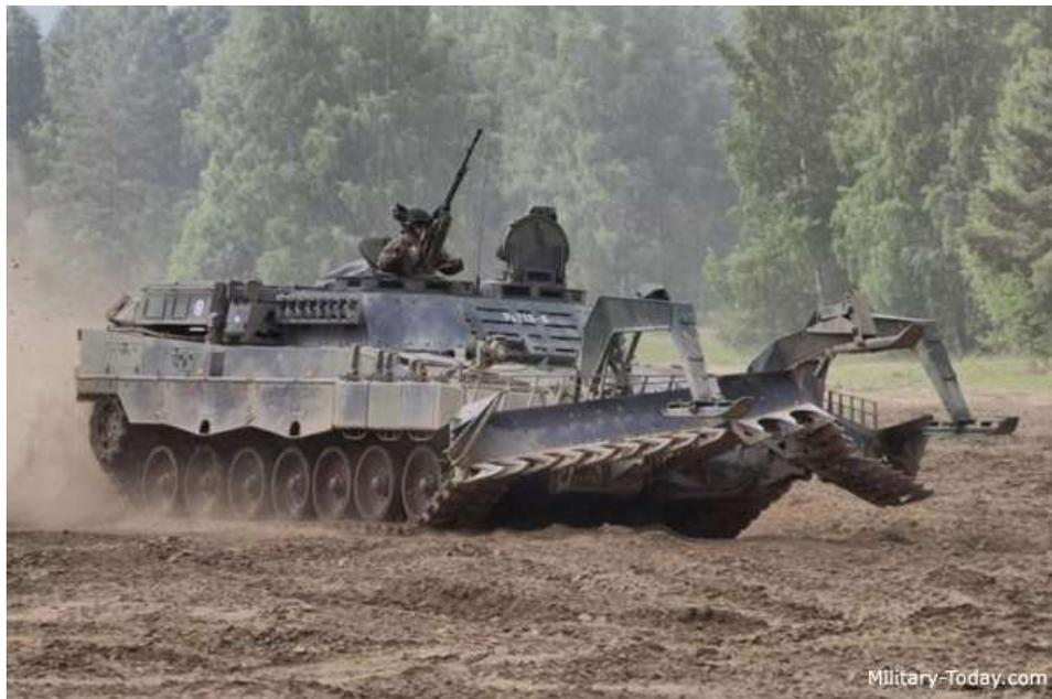
FIGURA 8 – Mine Clearing Roller System (MCRS)
