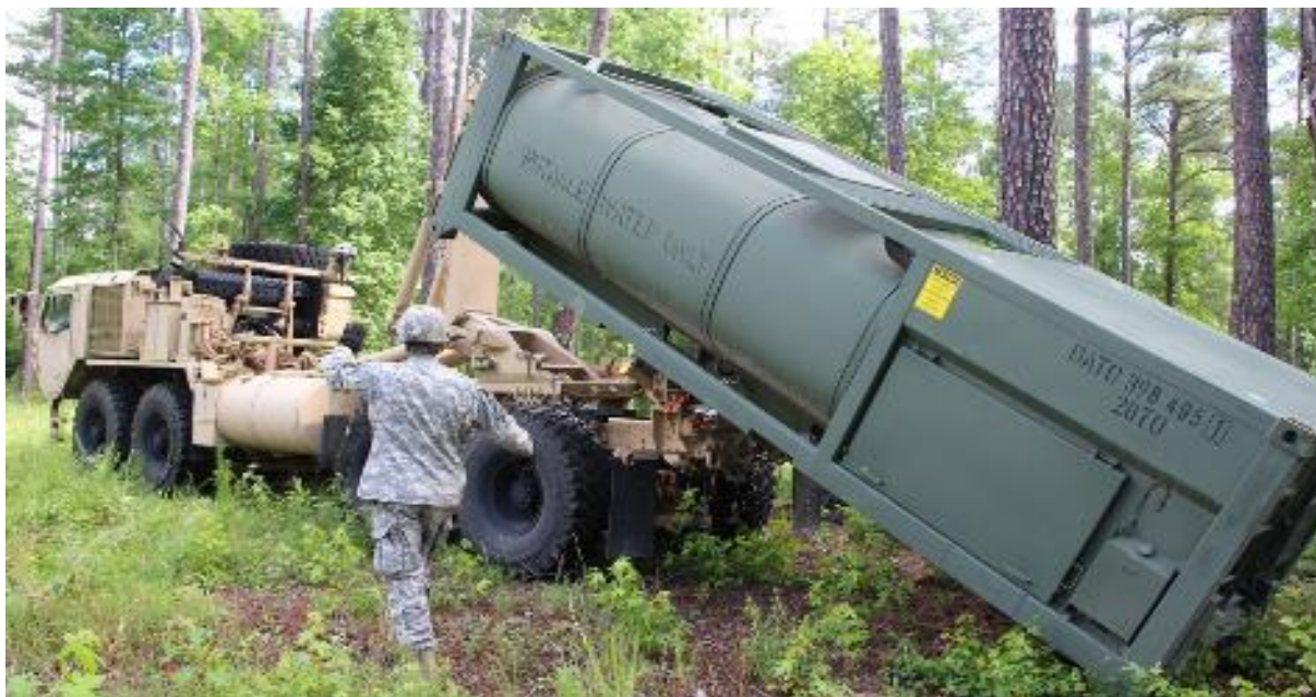
FIGURA 26- Water Tank Rack
