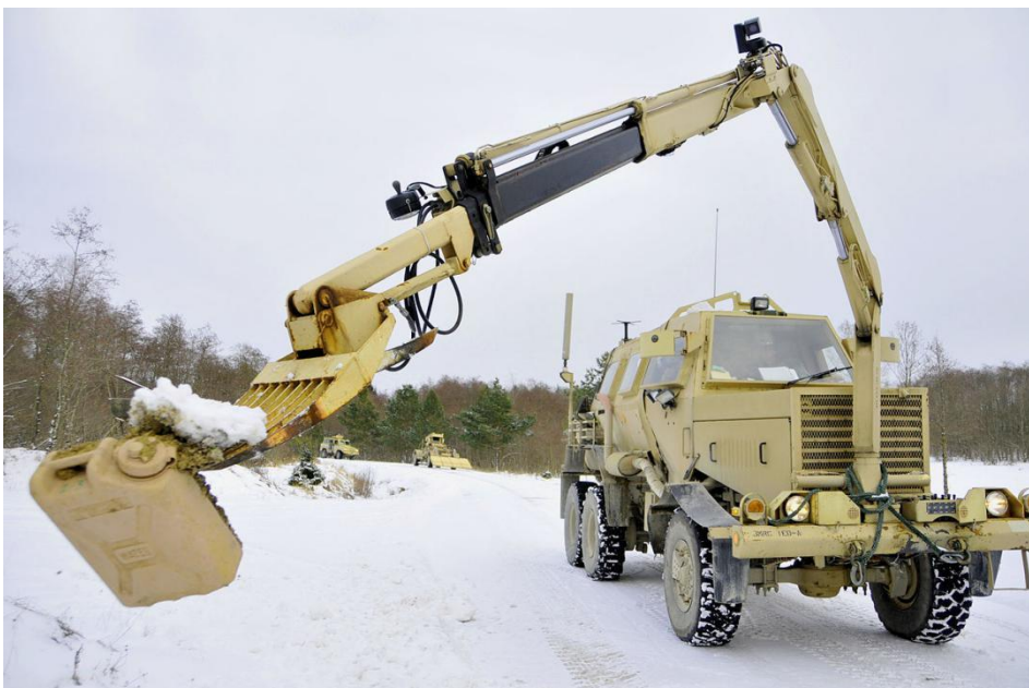
Fig 11 – Buffalo (mine protected vehicle) com braço manipulador
