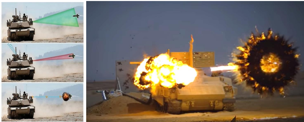
Figura 7 - TROPHY Active Protection System for AFVs
