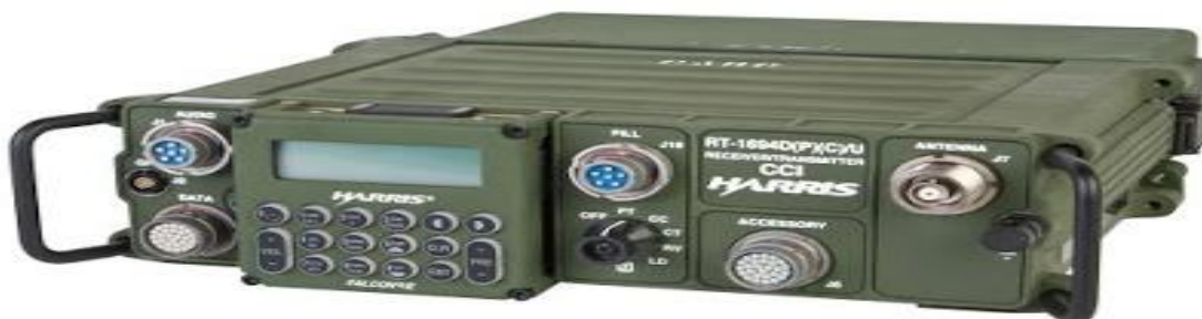
(FIGURA 1 – Transceptor Harris MPR 9600 (Falcon II) 3 )
